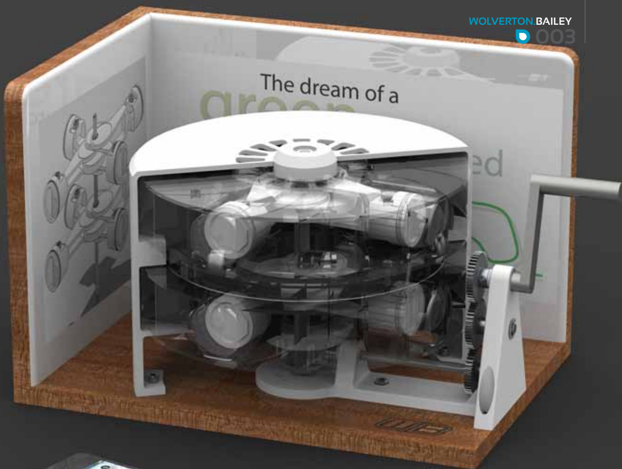
One Eight Scale 8 Cylinder Engineering Model: Built by California Polytechnic State University
